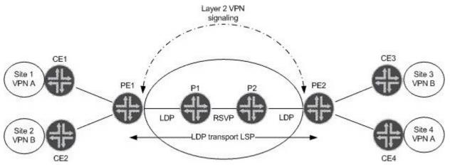
A LDP Layer 2 circuit is shown for VPN A and VPN B. LDP tunneling over RSVP is activated on P1 and P2.
