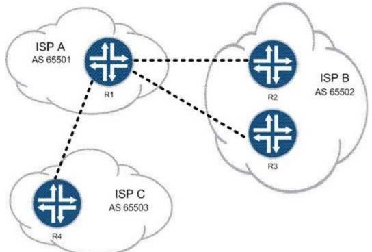
You work for ISP A. Customers of both ISP B and ISP C must be able to reach all of your customers, but your network must not allow transit traffic between ISP B and ISP C.
