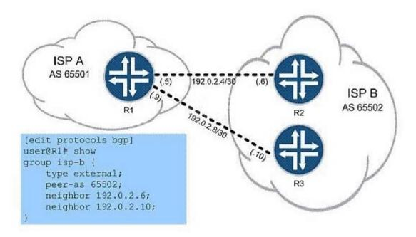
In the exhibit, ISP A is charged a higher rate for traffic sent to R2. You are asked to lower costs for ISP A by configuring R1 to send traffic to R3 whenever possible. What are two ways to do this? (Choose two.)
