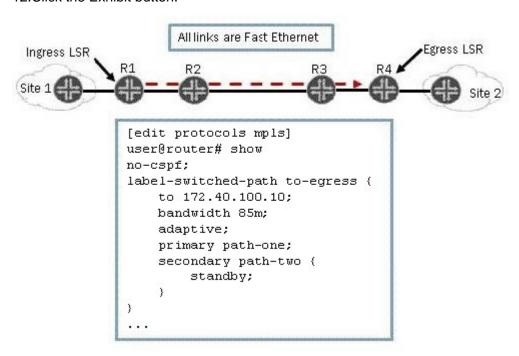
As shown in the exhibit, you have an adaptive LSP that requires 85 Mbps. The LSP is configured with a primary path and a secondary path in standby mode. All connections in the MPLS network are Fast Ethernet.
