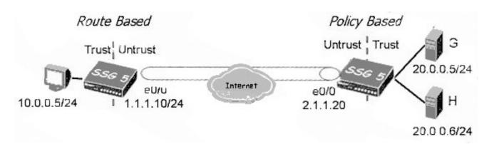
In the exhibit, the route-based VPN on the SSG 5 needs to configured to allow access only from your PC to Server G. The SSG 550 is configured with a policy-based VPN from Server G to your PC's host address.
