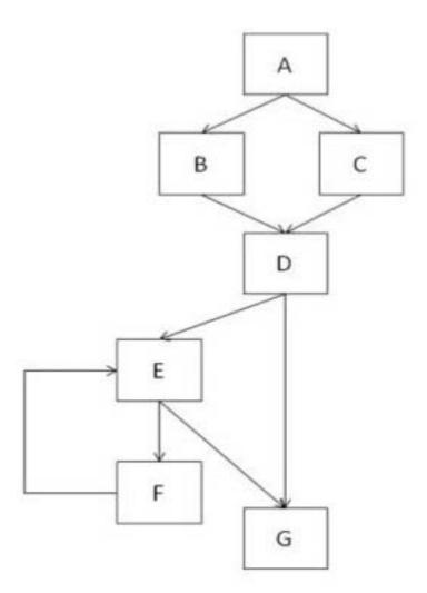
The following test cases have been run: -Test Case 1 covering path A, B, D, G
