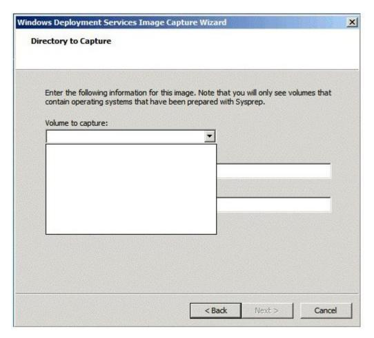
A.Start the reference computer from Windows Preinstallation Environment (Windows PE), and then run sysprep.exe /audit. Restart the computer by using Pre-Boot eXecution Environment (PXE).
