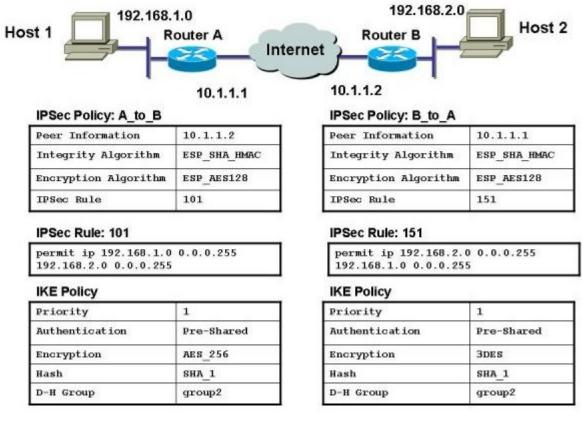
A. Router A is using a standard IP ACL (100-149) while Router B is using a Turbo ACL (150199).
