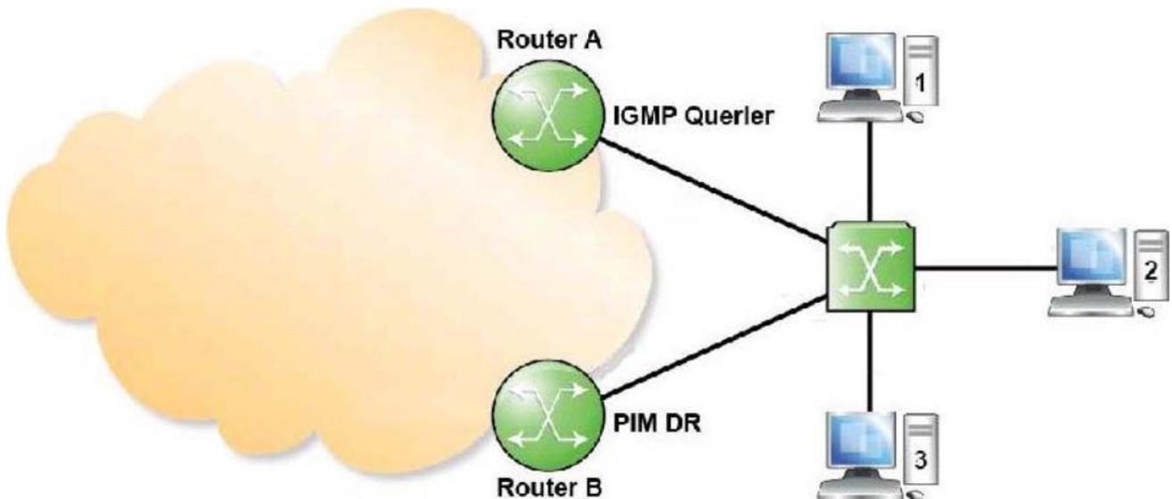
The switch is not igmp-snooping/proxy capable.
