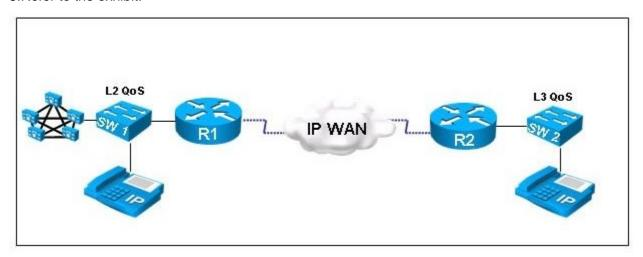
Traffic flows from the IP phone that is connected to SW1 to the IP phone on SW2. If the trust boundary has been extended to the IP phone on SW1, in what two places will traffic be marked and classified so that the proper QoS settings may be carried through the network? (Choose two.)
