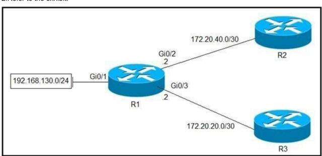
Which configuration configures a policy on R1 to forward any traffic that is sourced from the 192.168.130.0/24 network to R2?
